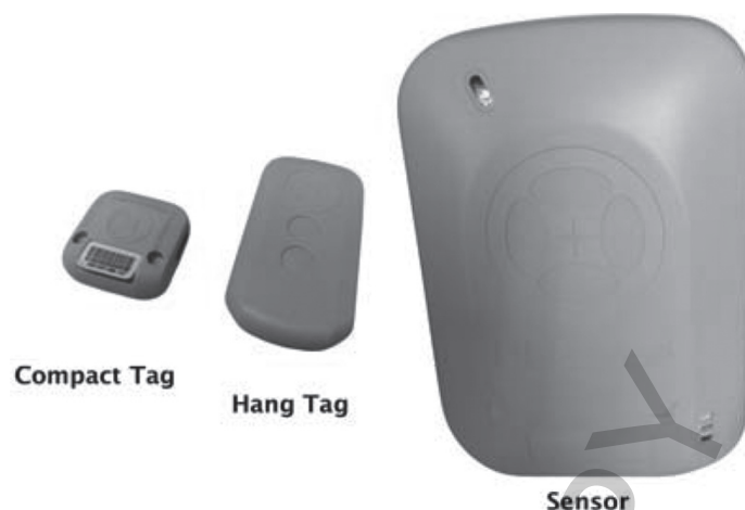
Fig. 1. UbiSense sensor (about 8" tall) and two tags used in the study (a wrist "compact tag" and "hang tag" worn around the neck). The tags emit an ultra-wide band radio signal that is triangulated by multiple sensors in the environment. The tags are worn by participants to track their location and movement in real-time.
