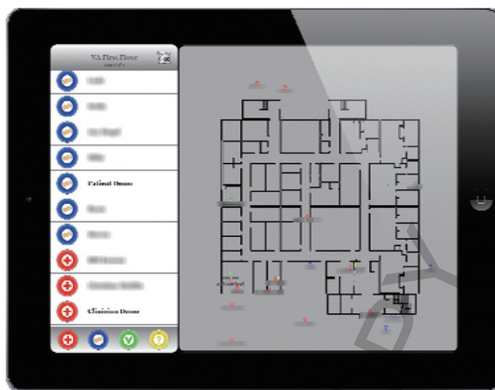
Fig. 2. The iPad Map application displays patient and staff location on a facility map. This application was incorporated into workflows and increased visibility and understanding of the real-time locating technology. (Colours are visible in the online version of the article; http://dx.doi.org/10.3233/THC-130738 )
